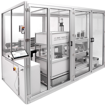
RMC 10000.5Y Robotic Mass Comparator
